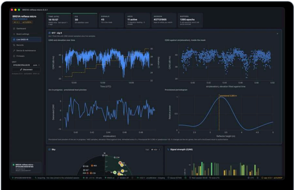
Arc inspector during a long pass: oscillation and provisional periodogram.
